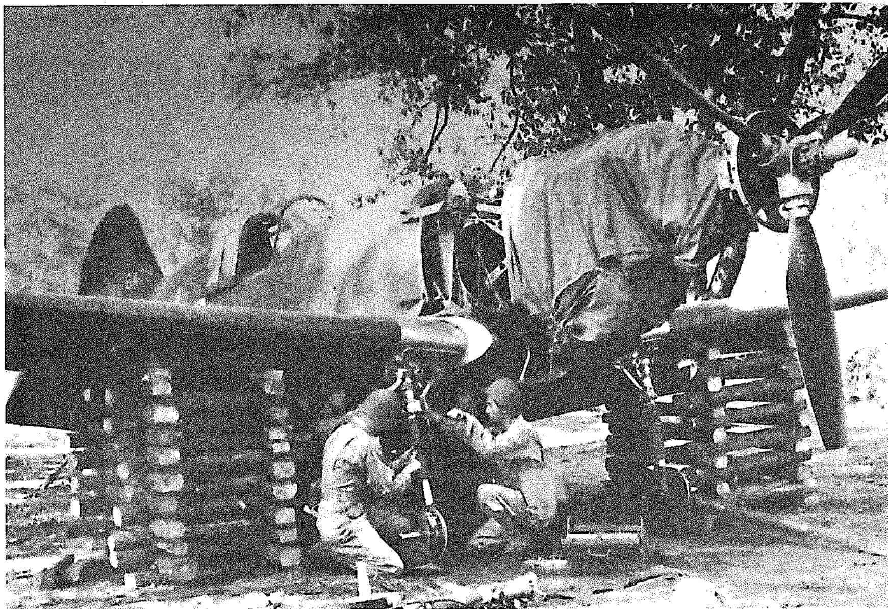
As part of the graduation field test trainees were required to replace a landing gear under simulated war-time conditions.
