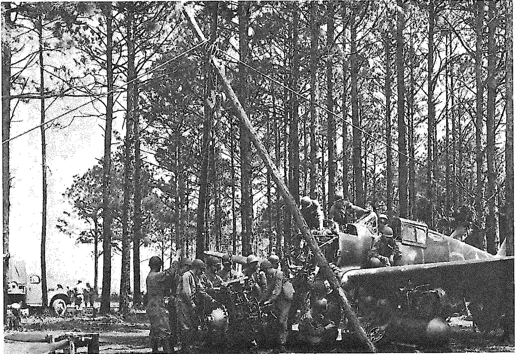
Students in the Graduation Field test training phase change an engine on a single-engine fighter plane under simulated war-time conditions.
